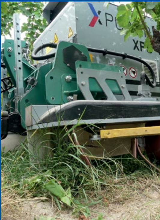
As a rear solution, the XPS is mounted on a hydraulic frame.
